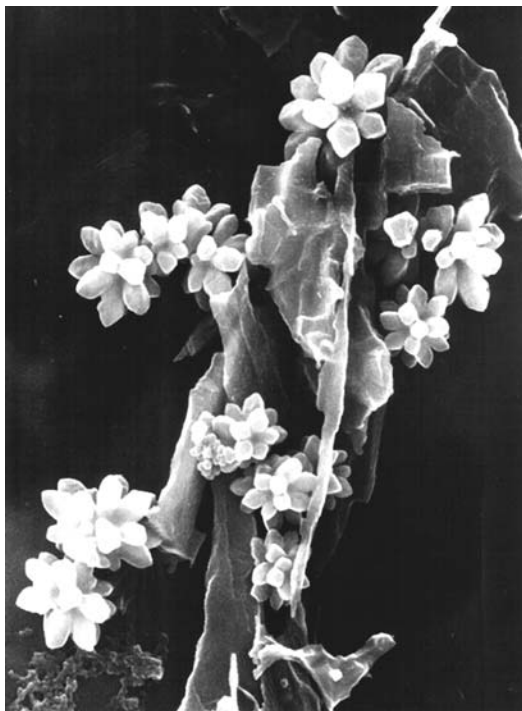
Figure 11. Icosahedral quasicrystals in a quenched Al/Mn sample. Sample by Ágnes Csanády (Budapest) and scanning electron micrograph by Hans-Ude Nissen (Zürich). Reproduced by permission.
